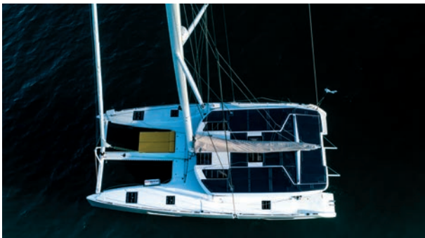
The deck layout of the New Windelo has been revised compared to the 54, and the coachroof has been lengthened, allowing for a greater area of solar panels.
