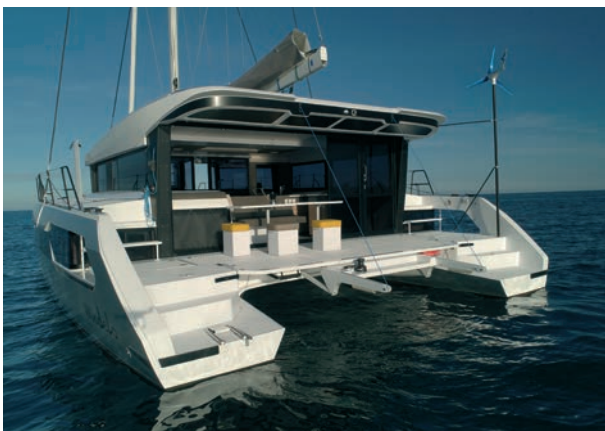
The aft cockpit is logically impacted by the nacelle being set further back: being very open, it is great in port and at anchor, but won't be much frequented in bad weather.
