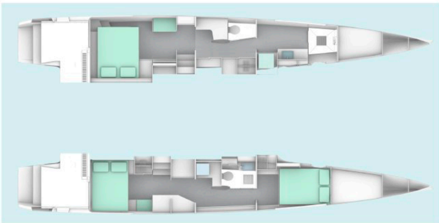
Windelo 54 - hulls plan for nacelle with L-shaped galley 1 master cabin, 1 office, 1 separated WC, 1 forward head 2 guest cabins, 1 central head, 1 central storage area
